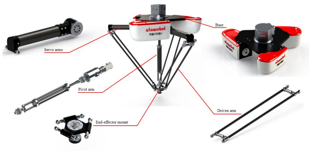
Figure 2-1 (D3P-1100-P0 Mechanism components)
